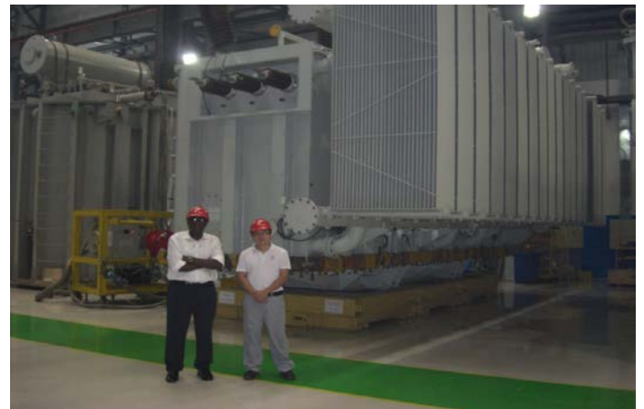
A 300 MVA Transformer for NIPP Project
